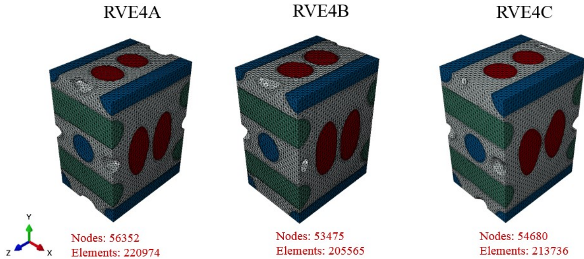
Fig. 3.II Finite element models of the RVEs of the 4DIN C/C composite.
